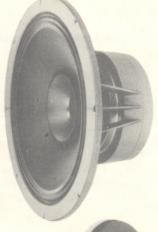
Nominal impedance: 8 or 15 Ohms Nominal power handling: 50 Watts Fundamental resonance: 56 Herz Sensitivity (96dB at 1m): 0.9 Watts Recommended enclosure volume for single unit: 80 Litres
