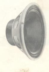
Nominal impedance: 8 or 15 Ohms Nominal power handling: 50 Watts Fundamental resonance: 85 Herz Sensitivity (96dB at 1m): 1.6 Watts Recommended enclosure volume for single unit: 50 Litres
