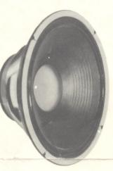
Nominal impedance: 8 or 15 Ohms Nominal power handling: 60 Watts Fundamental resonance: 70 Herz Sensitivity (96dB at 1m): 0.4 Watts Recommended enclosure volume for
